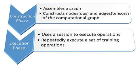
A *computational graph* is a series of TensorFlow operations arranged into a graph of nodes.
