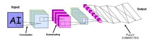
Figure 6-1. Layers in a convolution neural network
