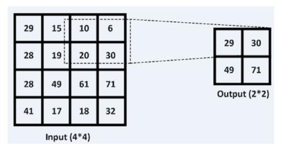
Figure 6-4. Maxpooling-reducing the number of pixels
