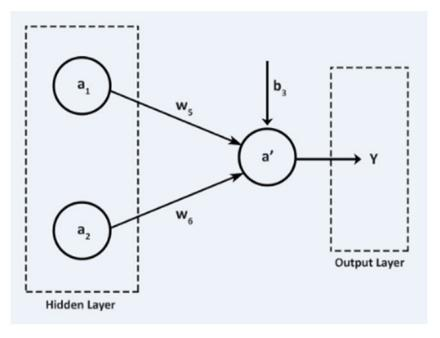
Figure 3-9. Forward propagation
