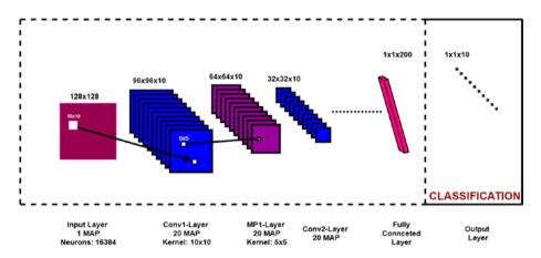
Figure 6-5. CNN Architecture for Classification
