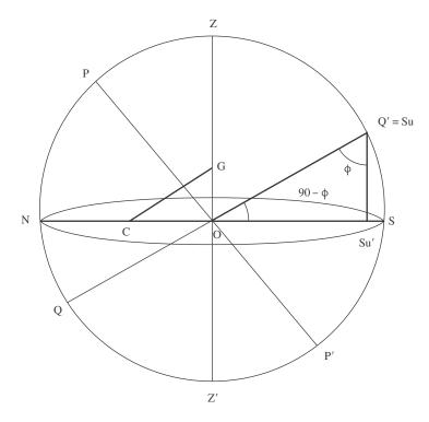
Figure 14.5 Latitude and co-latitude on an equinoctial day.
